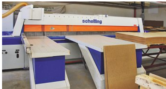
Backing board saw With this saw it is possible to mass-produce backing boards of every size.
