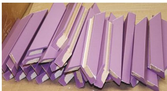
Staining The frame sections and their sawn edges are stained by hand to avoid untreated surfaces being exposed when the frame is assembled.
