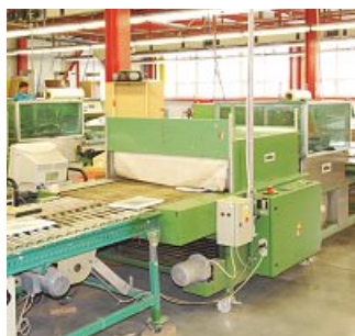
Shrink wrapping Since production began, around 59 million completed frames have been packaged using three shrink wrap machines.
