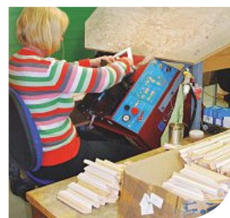
Finishing The frames are completed by the addition of their backing boards at several workstations.
