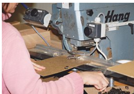
Fixing easy clips Easy Clips are mounted manually onto the backing board with a riveting machine.
